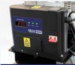
MAINS SUPPLY CONTROL BOX INITIATES START-UP FROM 16A SINGLE PHASE SUPPLY
